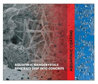
The chemistry in AQUAFIN-IC reacts with the concrete to grow crystalls which penetrate into the structure providing a permanent seal. The same chemistry will also work to self-heal static shrinkage cracks.
