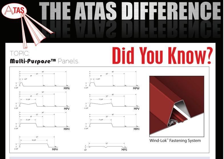
The <u>Multi-Purpose Panels</u> are structural panels with concealed fasteners that can be installed on open framing as well as to a solid substrate. Its <u>Wind-Lok®</u> attachment (positive fastening, without clips) saves time and money, while providing a variety of designs and looks.
