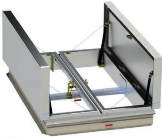
Type DSH-TB 60" x 96" (1524mm x 2438mm), Thermally Broken, R-20+ Insulation, Custom sizes available
