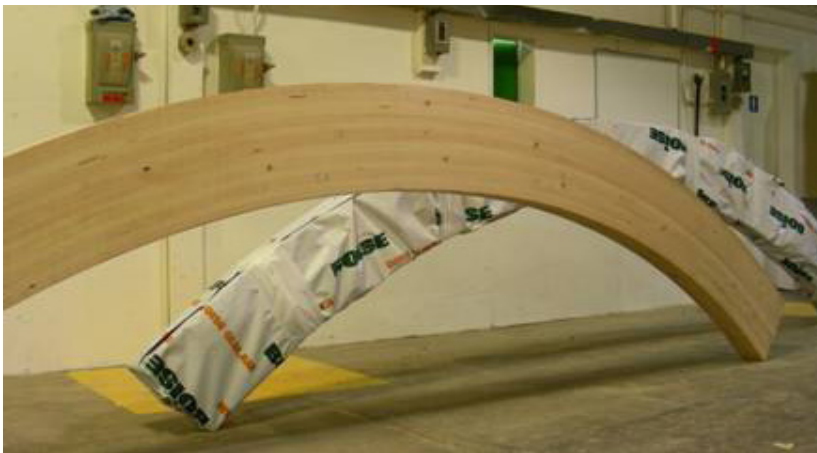
Finished Curved Beams
