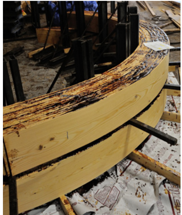
Clamping of Tight Radius Curve – ¾" Thick Laminations
