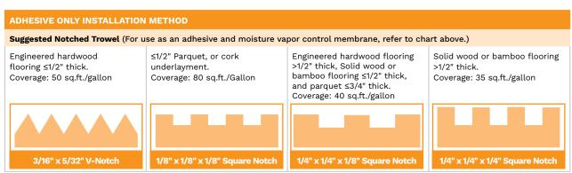
Trowel size is suggested to maximize coverage of adhesive. Periodically check coverage of adhesive during installation: >80% coverage and transfer to the back of the flooring is required for all engineered wood flooring; >95% coverage and transfer is required for all solid wood flooring or bamboo flooring products.
