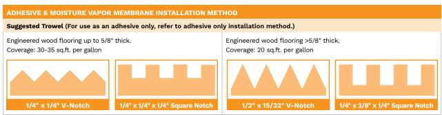
Trowel size is suggested to maximize coverage of adhesive. Periodically lift a board to ensure the following conditions are being met: 100% coverage of concrete substrate and 100% transfer to the back of the flooring product. Uneven subflooring may require the use of either a leveling/patching material or a larger V-notched trowel for proper coverage of adhesive.
