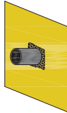
FILL TIGHTER GAPS WITH FRA-1 APPROVED SEALANT. FILL ROUGH GAPS WITH EXPANDING FOAM
