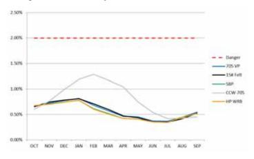
The simulation of the subject wall assembly using each of the WRB products indicates the exterior gypsum sheathing moisture content remains well below the 2% danger threshold. The wall assembly modeled with Fire Resist 705 VP very closely follows the behavior of the other permeable WRB products.
