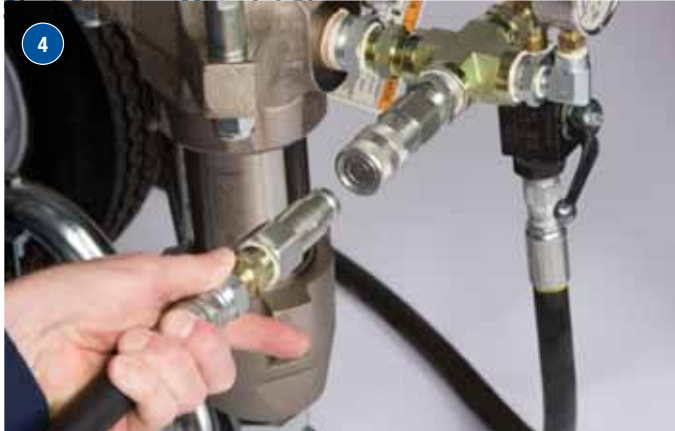
Connect jump hose to Graco pump.
