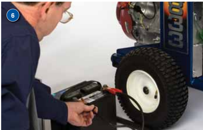
If pump does not have 12 V DC connection, connect clips to 12 V DC generator or 12 V DC battery. (GH 833 Model shown)
