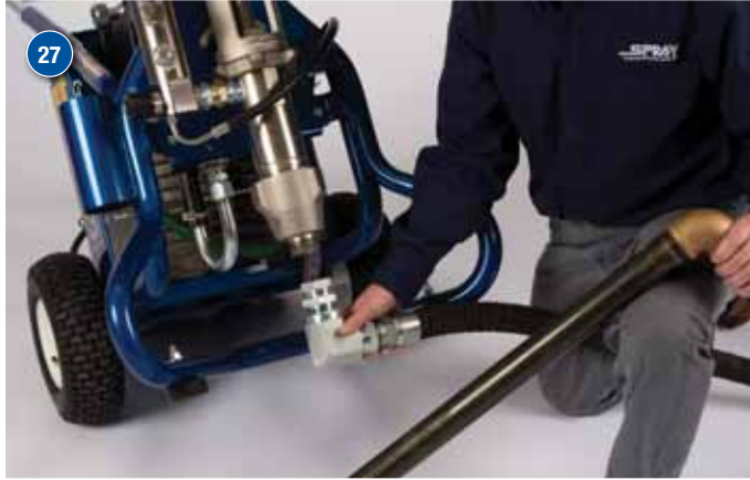
27 Disconnect drum siphon assembly.
