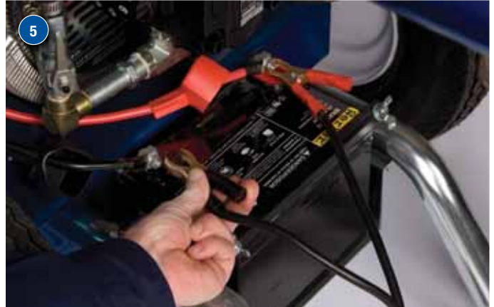
Connect alligator clips to 12 V DC on Graco pump. (GH 733 Model Shown)
