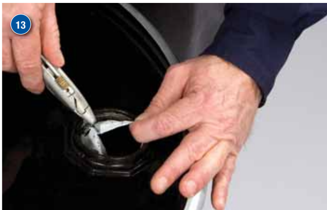
Unscrew bung cap on drum of Barriseal or Barricoat. Cut membrane that is visible through bung with utility knife.
