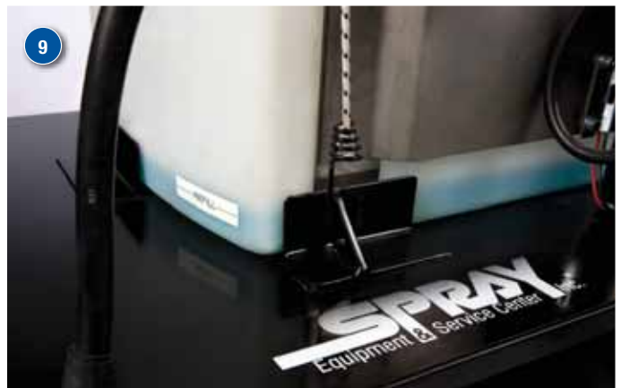
To re-fill tank, wait until Barricure solution is depleted to the empty line.
