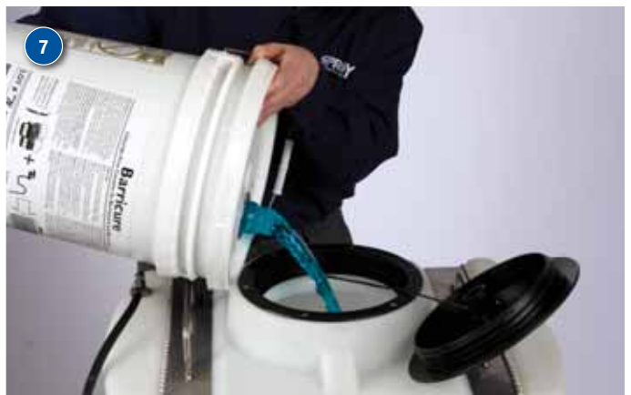
Pour full 5-gallon pail of Barricure into 25-gallon tank on Co-Spray Assembly.
