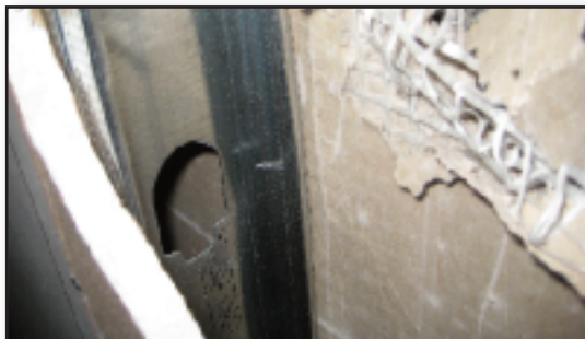
Soft body impact test using ViperStud.
