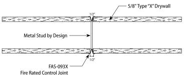
UL Systems available allowing installation on both or one-side of wall assembly. Consult UL System for details.
