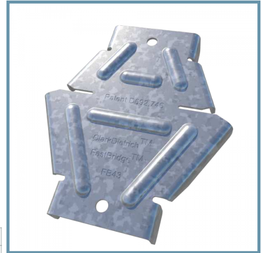
68mils (14ga) heavy-duty clip for use with 16ga to 12ga structural studs.
