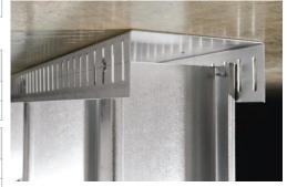
Calculating MaxTrak point load: Point Load (P) = (wind pressure PSF) x (spacing FT) x (wall length FT) / 2
