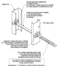
TYPICAL LATERAL BRACING DETAIL USING COLD-ROLLED-CHANNEL (CRC)
