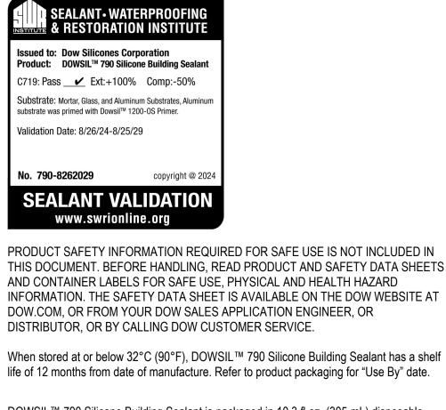
Packaging<br/>InformationDOWSIL™ 790 Silicone Building Sealant is packaged in 10.3 fl oz (305 mL) disposable<br/>cartridges that fit ordinary caulking guns, 20 fl oz (590 mL) E-Z Pak foil sausages that fit<br/>caulking guns, and also in 2.0 and 4.5 gal (7.5 and 17 L) bulk pails. It can be dispensed by<br/>many air-operated guns and most types of bulk dispensing equipment.
