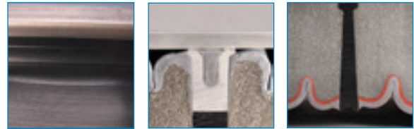
Heat-weldable TPR sidesheets (left) integrate with the deck waterproofing system. Watertight silicone bellows (center) sit under the trafficable coverplate. Spline (right) continues down through fire-retardant intumescent coating and silicone outer coating which line the SJS-FP-FR underside.
