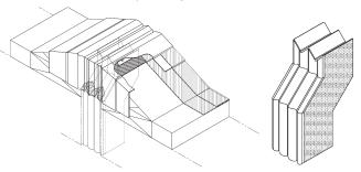
This single unit piece has factory-coated silicone bellows on the top and upper-back faces for integration with Seismic Colorseal in the wall and <a href="Horizontal Colorseal">Horizontal Colorseal</a> as a secondary seal and insulator across the roof. The silicone-coated top side of the closure is shaped to match the underside of the RoofJoint extrusion.
