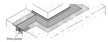
Strain-relieving shear-pockets, an Emseal innovation, allow for full movement-range capability, free of tensile stress. **Shear pockets** are ideal at jogs around columns, at tees, and other high-movement transitions.
