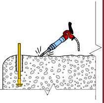
2. Anchor bolts should be prepared with at least 10 bolt diameters embedded for anchoring and at least 12 bolt diameters for free stretch. The free stretch length of the bolt must allow stretch of the bolt and prevent bonding of grout to the bolt.
