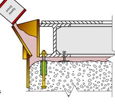
9. After recommended cure time, based on exposure temperature, has elapsed, remove formwork and alignment devices. Tension anchor bolts. Equipment start up may now commence.
