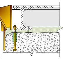
7. Pre-condition the Chockfast components, mixing equipment, and application area to 65°-95°F (18°-35°C).
