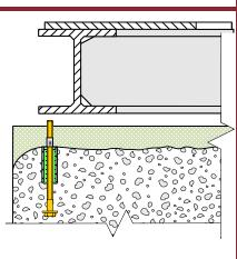
5. Install and align equipment on foundation using removable alignment devices, such as jacking screws. Screws should be well coated with a non-melt grease and land on a rounded leveling plate, anchored to the concrete with a structural adhesive, such as Phillybond #6.
