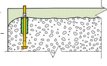
4. All bonding surfaces should be well cleaned and free of any dust, dirt, oil, water, or other residue. Any steel surfaces should be near white bare steel or coated with a high quality epoxy based primer.
