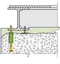
6. Nuts should be hand tight on anchor bolts to prevent floating of base. Construct leak-free formwork to place epoxy grout. Head boxes are recommended to provide hydraulic head pressure and aid installation. Coat forms with 3 coats of paste wax to prevent bonding.
