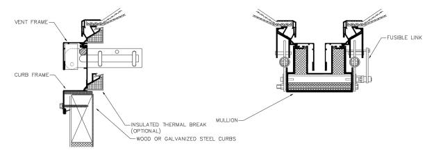
• Smoke Vents shall operate by a fusible link with a minimum temperature rating of 165 °F (74 °C). The fusible link mechanism with gas shocks shall include an exterior manual release cable for testing.
