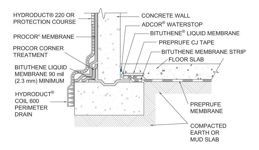
NOTE: THE FOOTING KEYWAY SHOULD BE FORMED TO CREATE A REGULAR AND UNIFORM SHAPE ALLOWING PROPER DETAILING OF THE BITUTHENE LIQUID MEMBRANE.
