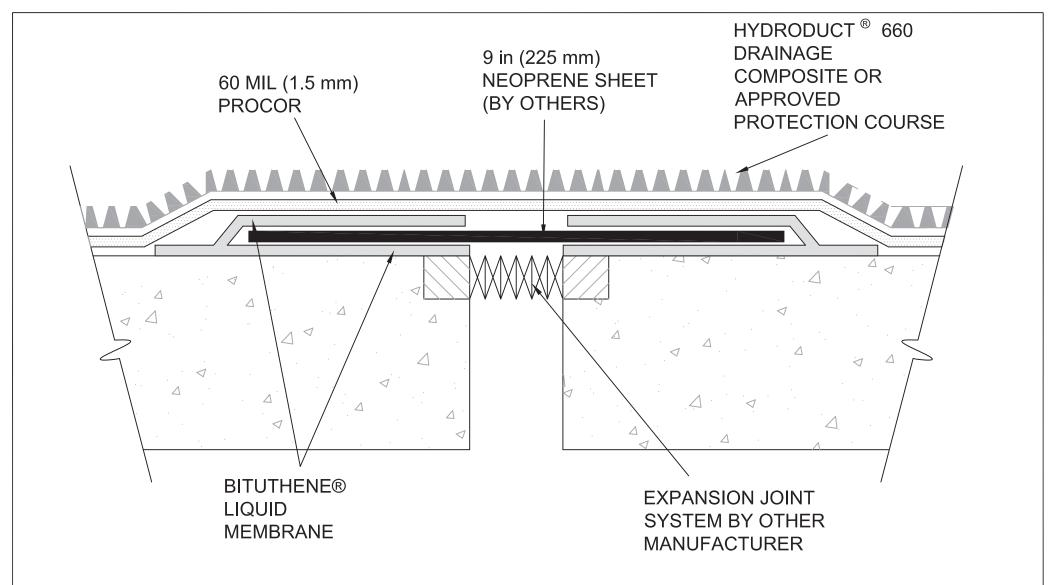
NOTES: - FOR JOINT WIDTHS UP TO 2 IN. (50 mm) WITH A MAXIMUM MOVEMENT OF 1 IN. (25 mm) MOVEMENT - A WATERPROOF EXPANSION JOINT SYSTEM BY OTHERS MUST BE SELECTED FOR THE WIDTH AND EXPECTED MOVEMENT OF THE JOINT, SEE TECHNICAL LETTER 11 FOR ADDITIONAL INFORMATION.
