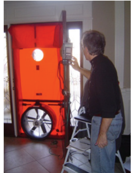
Figure 17: Blower door testing
