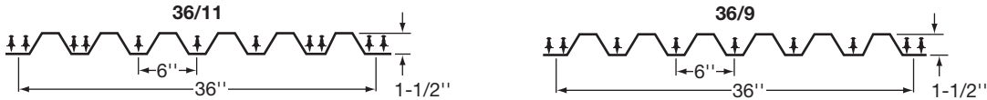
Figure 18 — Allowable Stress Design (ASD) – Allowable diaphragm shears, S_{ASD} , (plf) and stiffness factors, G' , (kips/in.) for standard 1-1/2" deep flutes, 6" center-to-center deck ( F_y \geq 50 ksi; F_u \geq 65 ksi) installed with Hilti X-HSN 24 fasteners with 36/11 or 36/9 end and interior support fastener patterns 1,2,3,4,5
