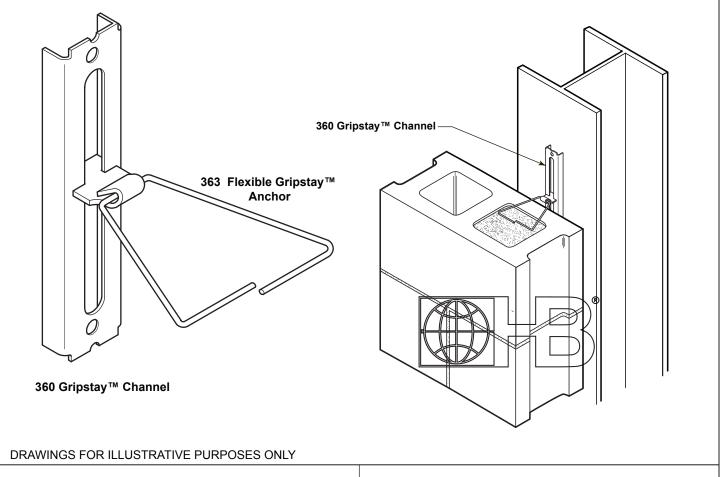
The **360 Gripstay™ Channel** welds onto steel web or flange to accept any type of Gripstay™ Anchor.
