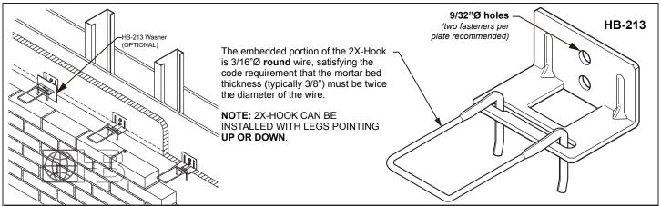
Hohmann & Barnard's 2X-Hook has been tested and designed to withstand over 200-lbf, in tension or compression, at maximum allowed offset (TMS 402/602-16 12.2.2.5.5.4) of  $1\frac{1}{4}$ " (disengagement of the pintle from the veneer anchor). These results exceed BIA recommendations and the capabilities of standard "round wire" hooks/pintles by over 100%, while maintaining the ASTM A1064/1064M wire specification.
