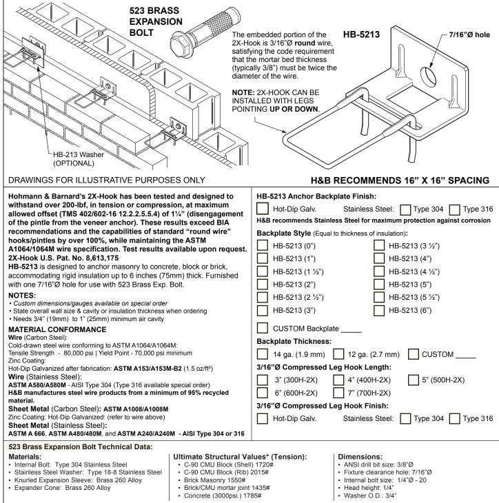
\* Full 1" Embedment. \* The ultimate structural values listed above are ultimate load capacities, which should be reduced by a minimum safety factor of 4.0 or greater to determine the allowable working load.
