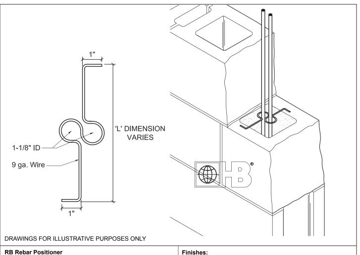
For positioning rebar in center of block. The Z-shaped wire bridges cell of block while bends rest on shell.
