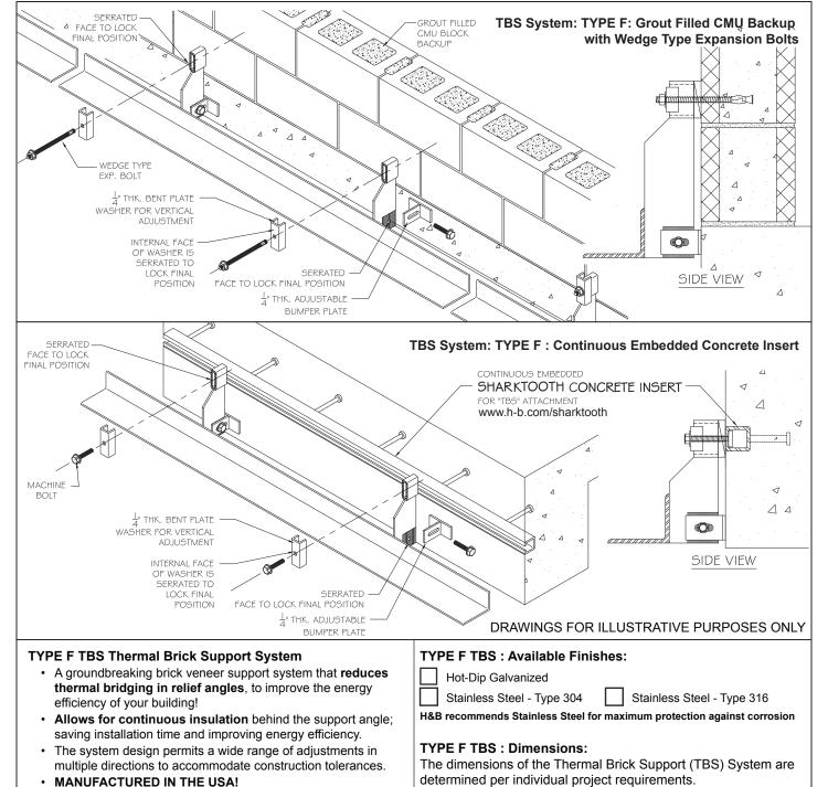
**MATERIAL CONFORMANCE** Carbon Steel: ASTM A36
