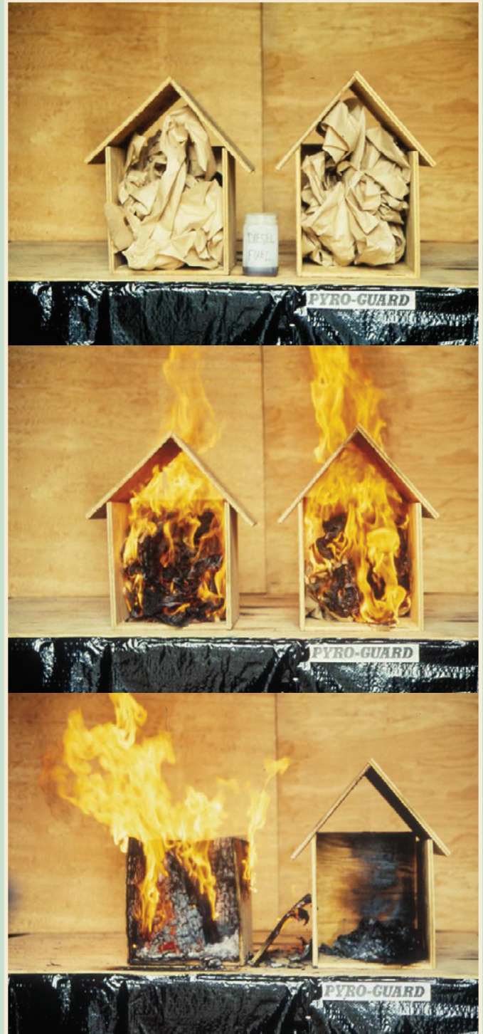
The identical contents within an untreated wood structure (left) and a PyroGuard™ wood structure (right) were set on fire. After 15 minutes, the untreated structure became fuel and continued to burn. The PyroGuard™ structure self-extinguished after the combustible contents were consumed, demonstrating FRTW does not add fuel to the fire.
