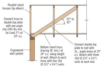
\* Load 2 value from Lateral Connections—Angle Clips table below.
