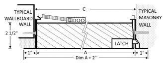
CEILING INSTALLATION (Side View) Use "C" Dimension for Stud to Stud or Masonry Installation Without Wallboard Liner
