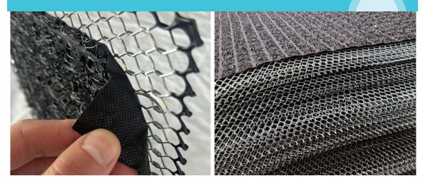
LathNet is a metal lath and drainage plane system that provides a continuous drainage plane between the lath and weather resistant barrier. The Masonry Advisory Council recommends that in exterior adhered masonry wall systems, a drainage mat be installed to drain any water that has penetrated to the flashing. A galvanized expanded metal lath, or diamond mesh, should be attached atop the drainage mat.
