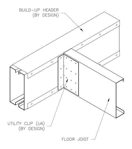
UTILITY CLIPS (UA) - JOIST TO HEADER CONNECTION
