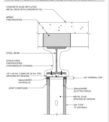
3/4" NOMINAL GAP Marino\WARF HOTROD XL JOINT COMPOUND Marino\WARE SLOTTED METAL STUD SPACING BY DESIGN
