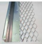
USE: As a plaster stop and as exposed trim around window and door openings. Can also be used at the junction or the intersection of plaster and other wall or ceiling finishes. Zinc should be used for exterior applications. Available with weep holes.
