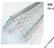
USE: It is galvanized steel and has full 3-1/8" flanges. It is easily adjusted for plaster depth on columns and is ideal for structural tile corners with rough masonry. Double X Corner Bead has perforated stiffening ribs along the expanded flanges.
