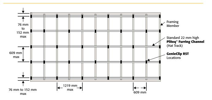
Wall or Ceiling Framing at 16" o.c. **GenieClip RST** at 48" o.c., furring at 24" o.c. 1 or 2 Layers of  $\frac{5}{8}$ " Gypsum Board
