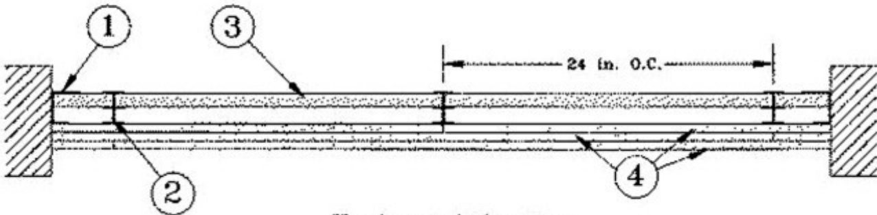
Horizontal Section System H - 3 Hr.
