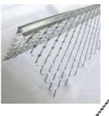
**USE**: Available in zinc or galvanized steel. Wide expanded flanges are easily flexed. Preferred for irregular corners. It provides increased reinforcement close to the nose of the bead. Zinc should be used for exterior applications.
