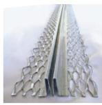
USE: To relieve the stresses of expansion and contraction in plaster or stucco. It is available in zinc or galvanized steel. Zinc should be used for exterior applications.
