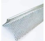
USE: Galvanized steel, used with one-coat or two-coat veneer systems to provide 3/32" grounds. With 1-1/4" fine mesh flanges, either stapled or nailed, provides an effective plaster key and eliminates shadowing
