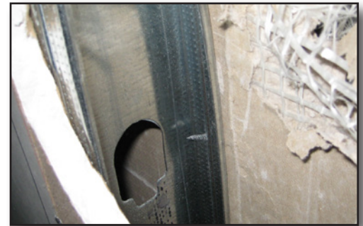
Soft body impact test using ViperStud.
