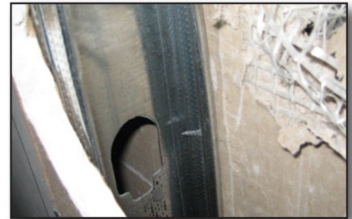
Soft body impact test using ViperStud.
