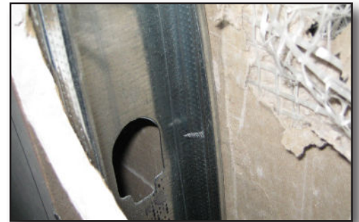
Soft body impact test using ViperStud.
