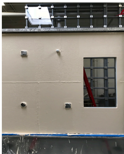
ASTM 2357 Test Panel - Completed
