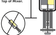
Tilt Gun Down and **Squeeze First** 2-3 Shots of Material into A Disposable Cup, Etc.
