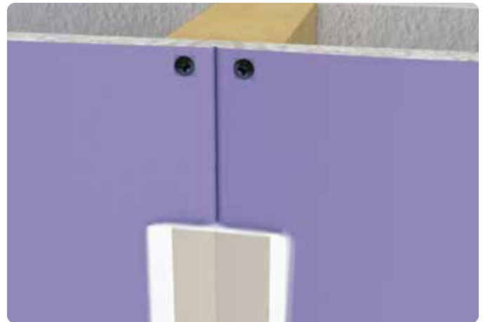
1 All joints and interior angles have tape set in compound.
