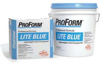
Designed for use in finishing gypsum board joints, spotting fasteners and finishing cornerbead. ProForm® Lite Blue Joint Compound is a lightweight, vinyl base ready mix joint compound. Approximately 30% lighter than a conventional ready mix, Lite Blue Joint Compound pulls and sands easier and reduces shrinkage by up to 33%.
