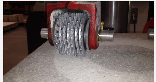
The ASTM C779 Procedure B uses steel dressing wheels to test the abrasion resistance of concrete surfaces. (Source: Nelson Testing Laboratories)
