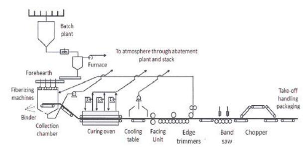
The diagram above is representative for the manufacturing of bonded fiberglass insulation product. There are no significant process differences between locations.
