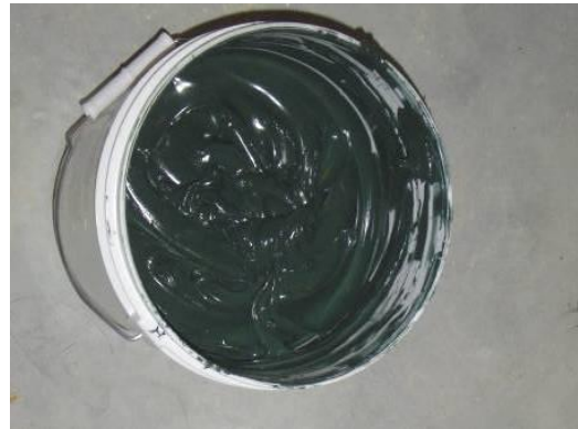
Photo #16 – Fully mixed sealant
