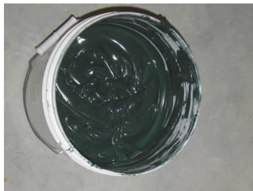
Photo #16 – Fully mixed sealant
